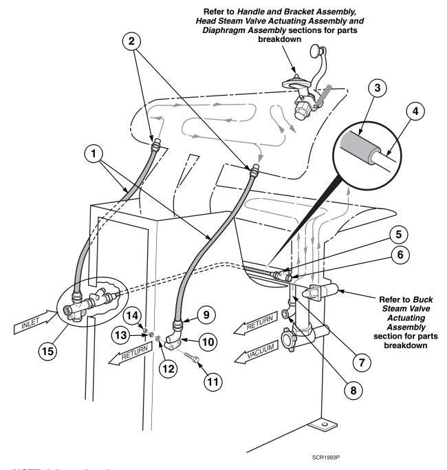
NOTE: Inlet and outlet are shown on a right hand machine. Left hand machine is a mirror image.
